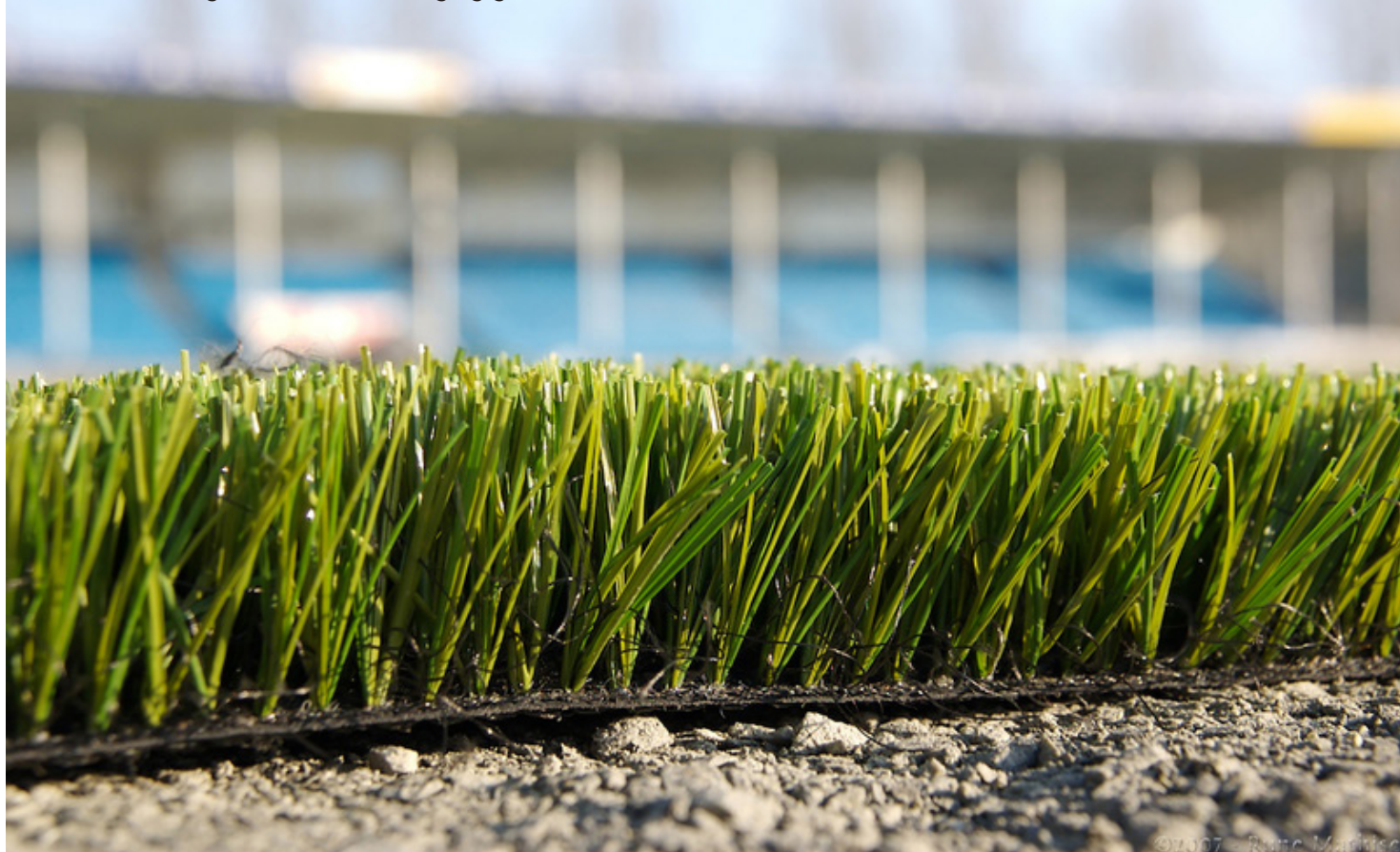
Figure 1. Paved and artificial surfaces – known to landscaping professionals as "hardscaping" – reduce the possibility of water infiltrating the soil and recharging groundwater. Photo Wikimedia.
